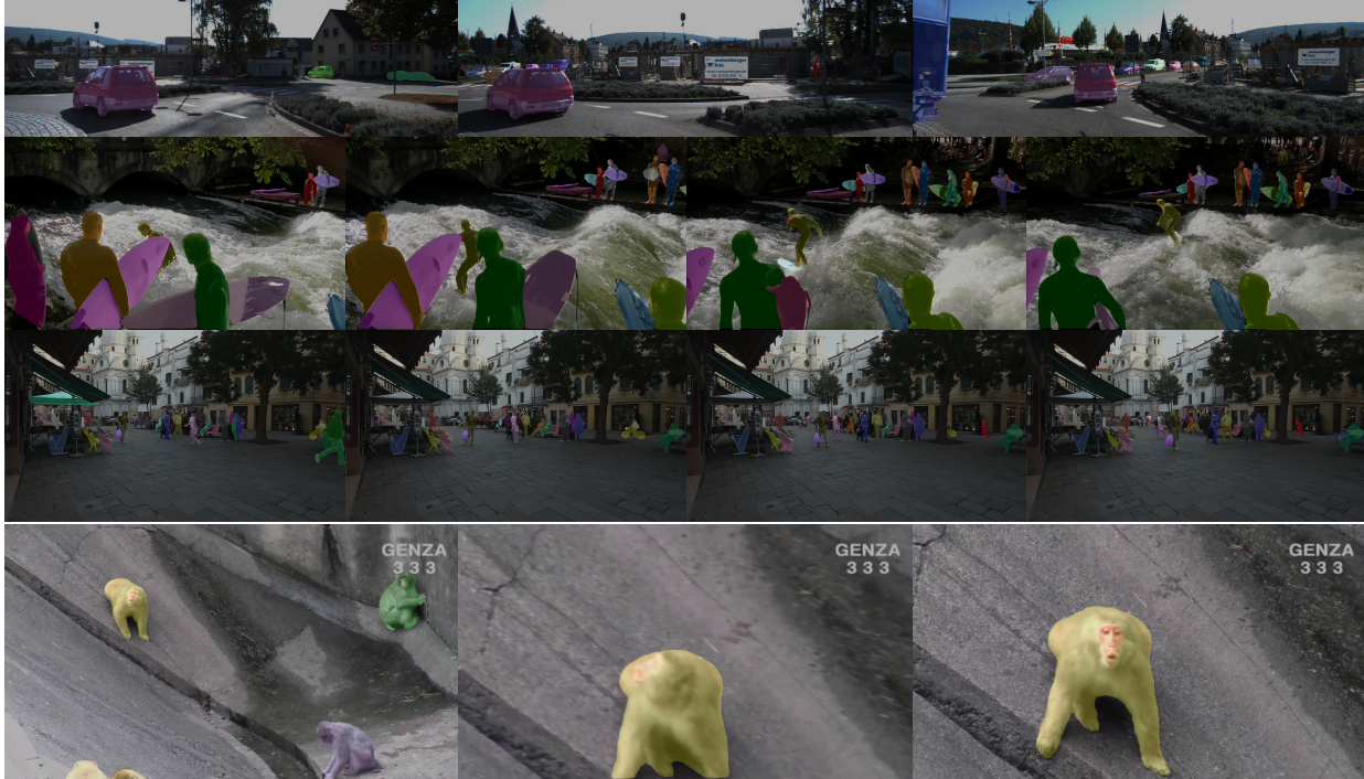
Figure 2. Qualitative results of the proposed SIA. 1st row: KITTI MOTS (moving camera); 2nd row: DAVIS Challenge Un-supervise (moving camera); 3rd row: MOTS Challenge (static camera); 4th row: TAO (moving camera, zoom in).
